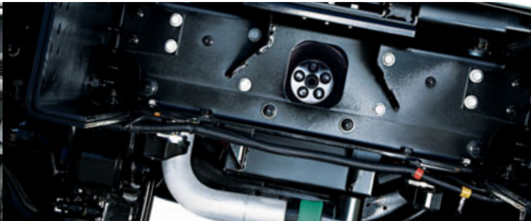
Available radiator placement above the frame-rails provides for uninterrupted front engine power take-off (FEPTO) mounting below the radiator
