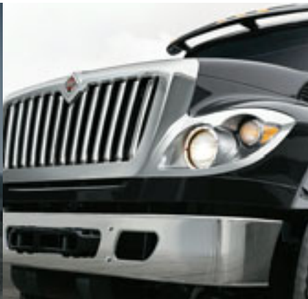
Three-piece hood keeps repair costs down in case of an accident
